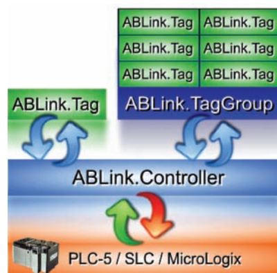
Figure 2: Only three primary classes of .NET code manage all communications with the PLC.
