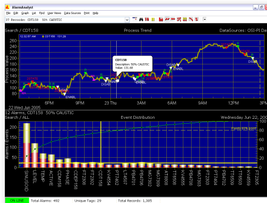
Fig 1 Some of the high level on-line views showing equipment fault rates, durations and operator actions fully integrated with continuous plant data.
