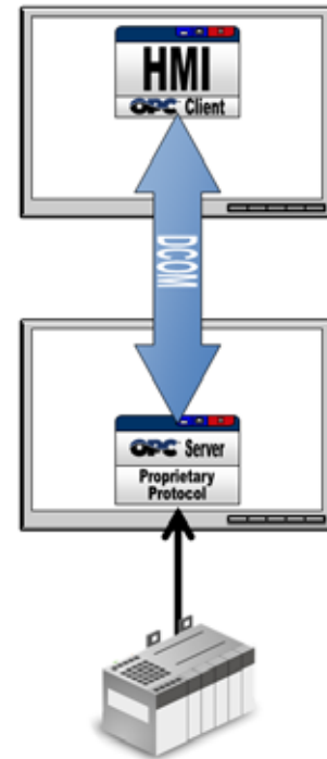
Image 2: OPC initially relied on DCOM for data transportation. DCOM is a highly secure and fast API from Microsoft that provides applications with services for authentication, authorization, and encryption.
