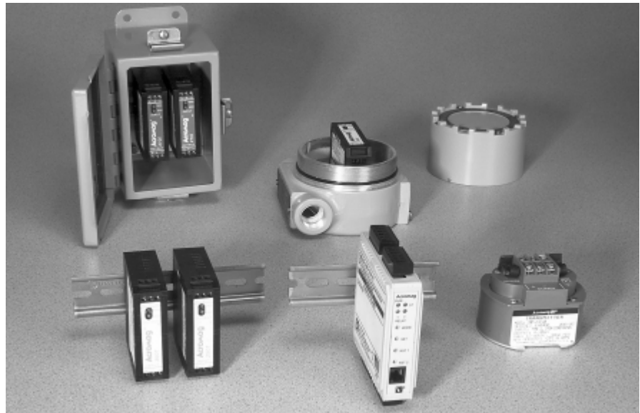
Signal conditioners are available in many formats: hockey-puck, rack-mount, DIN-mount, wall-mount, etc.
