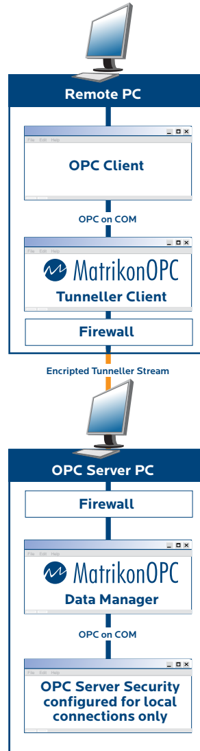
Fig 3. Tunnelled OPC using MatrikonOPC Tunneller
