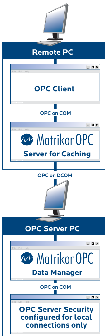
Fig 2. "Push" Architecture using MatrikonOPC Data Manager and OPC Server for Caching
