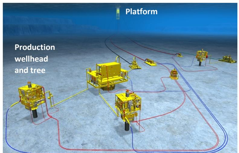
Subsea production tree on top of wellheads piping oil or gas to topside production platform for processing and storage.
