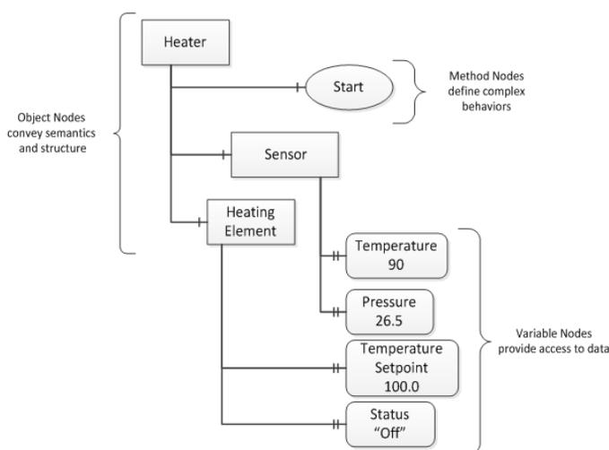
OPC UA provides a framework that can be used to represent field devices, for example. A heater (or other object like a motor, pressure transmitter, valve) can be represented as a heater object. The heater object can have subcomponents like a heating element object. The heater object can have method objects that define behaviors for the heater object like start heater. The heater object can have variables like temperatures and pressures that can be read/write values.
