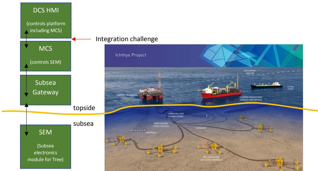
Imagine all the integration effort required for a seemingly simple action from the DCS like "open valve" that requires an orchestrated interaction between DCS, PLC (MCS), and the valve on the ocean floor.
