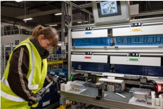
*Thanks to the Poka Yoke controller, existing technology, like a digital torque wrench in this case, can easily be integrated into the error-free process.*
