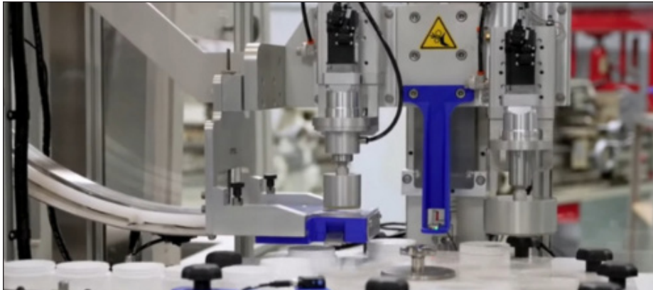
Figure 2. Balpack, Mitsubishi Electric and HPE Automation developed a precise torque control system for capping small bottles.
