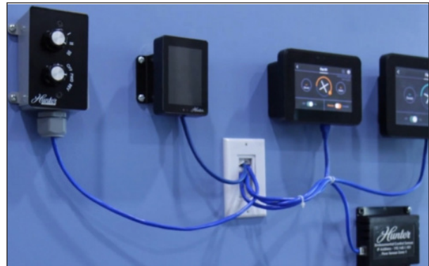
Figure 1. At Hunter Fan, operator interfaces were replaced with glass touchscreens powered by PoE.
