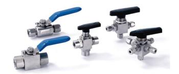
MET-LOK Ball valves are available in size range from 1/8" to 1" with NPT, BSP, BSPT male/female end connections. These valves are design for application on instrument lines, gas sampling lines, pneumatic systems, pilot plants, analyzer labs etc. These valves perform on/off functions
