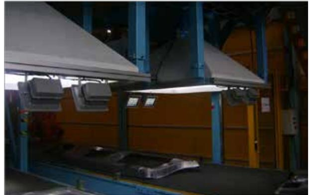
*In the first phase of the assembly process, Teledyne DALSA's GEVA 1000 vision system, with two Genie high-resolution 2MB 1600x1200 cameras, completes two distinct inspections of each vehicle part: first to identify the type of part and second to assess the part to ensure accurate positioning of the robotic arms that will lift and move it into production.*
