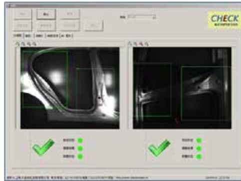
*Teledyne DALSA GEVA 1000 includes Sherlock software, which uses its Search Tool – one of the quickest and most accurate pattern-matching tools in the industry – to analyze the images to identify the coordinates of all positions and ensure alignment. Sherlock's calibration capabilities and alignment algorithm parameters minimize barrel distortion and help ensure marks can be seen clearly so that lifting positions are accurate.*
