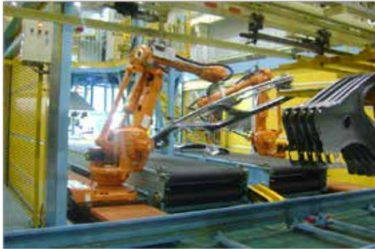
*With guidance from Teledyne DALSA's GEVA 1000, which communicates via built-in I/O and RSS232 industry-standard protocols, specially designed robotic grippers lift the vehicle part onto the assembly line automatically. Thanks to vision guidance, the robotic grippers can now move a part every two minutes, increasing production speed by six times overall.*
