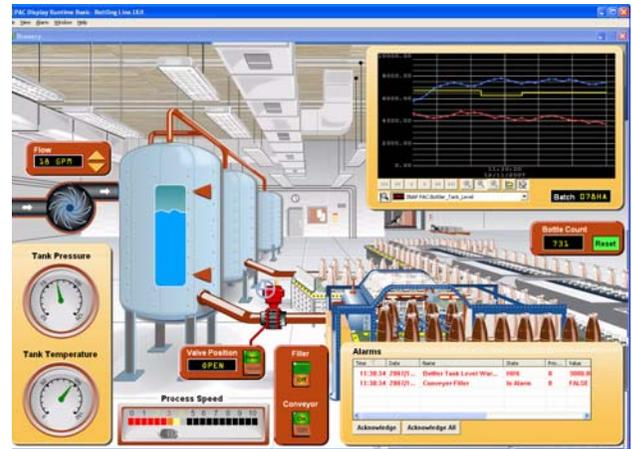
PAC Display HMI development software uses the same database of I/O points and variables as PAC Control.
