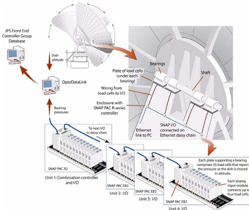
2. In electrical and electronic engineering, a daisy chain is a wiring scheme in which, for example, Device A is wired to Device B, Device B is wired to Device C, Device C is wired to device D, and so on. Daisy chains may be used for power, analog signals, digital data, or a combination thereof.
