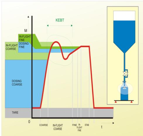
Figure 1: Spreading during fill
