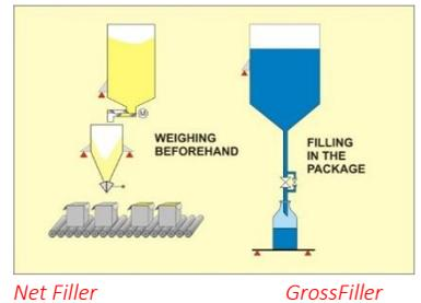
In accordance with the e-mark ruling, filling packages of  $\leq 10$ kg is done based on average weight.
