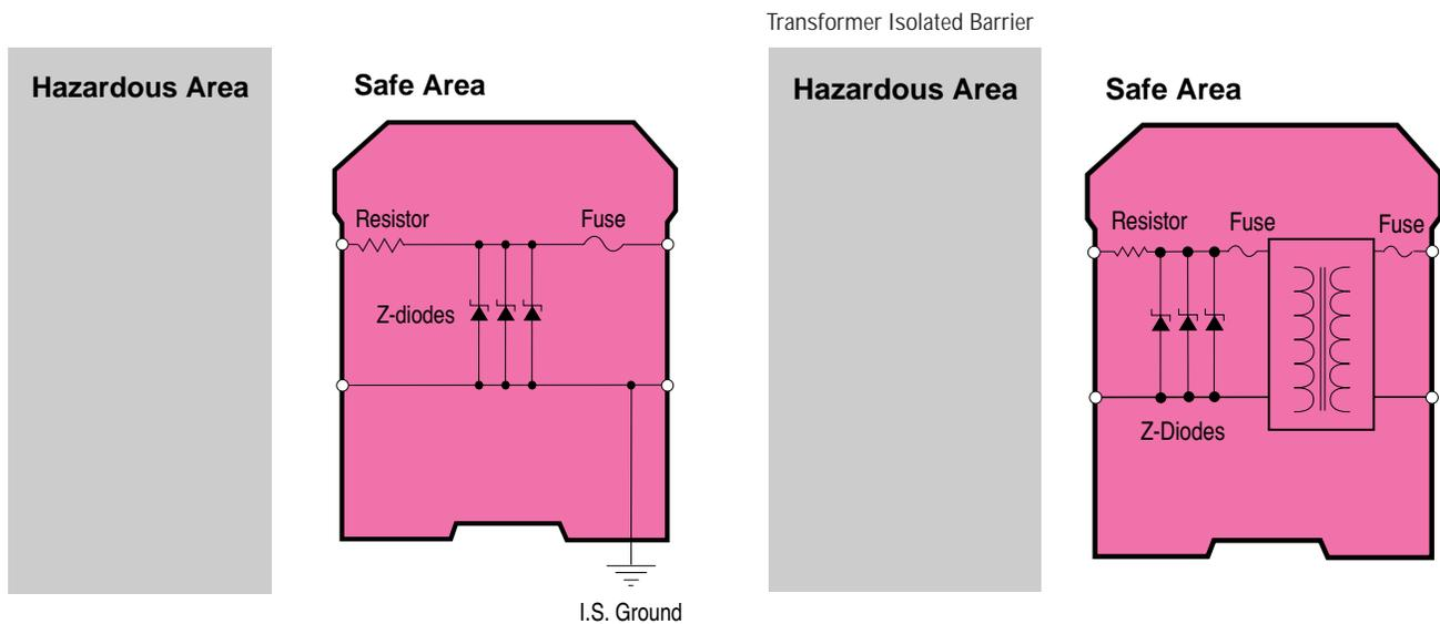
Because of these considerations, we have designed a different type of barrier known as a Transformer Isolated Barrier (TIB). It is designed to address each of the disadvantages of zener barriers.
