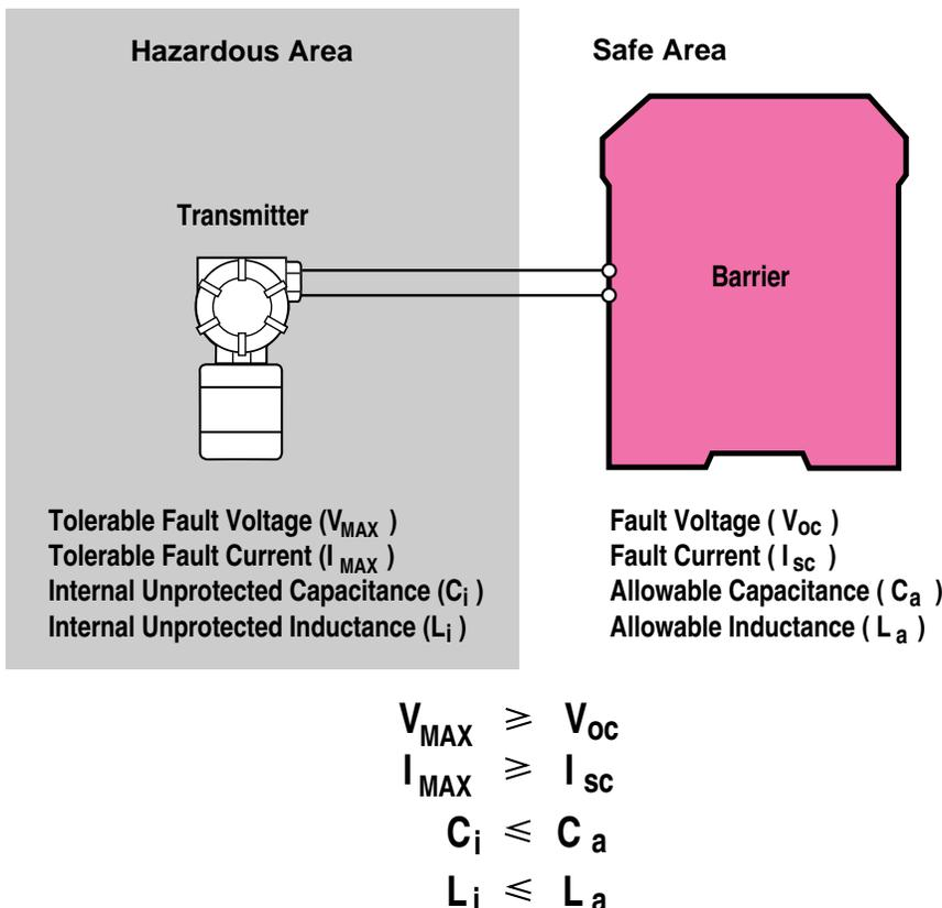
The safety barrier is given the following entity parameters:
