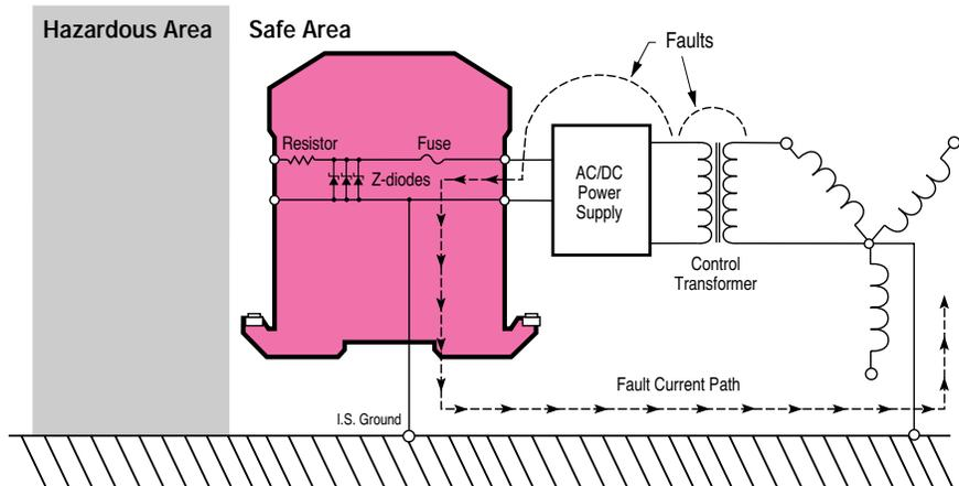
In a TIB, the fault current will flow through the primary of the transformer. Once the current has reached a sufficient level, the fuse will open, preventing the fault condition from reaching the hazardous area.
