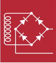
Some I.S. solenoid manufacturers go a step further when installing diodes in their valves. They are installed as full wave bridge rectifiers which give the additional advantage of non-polarity sensitive valves. The diodes in series cause an additional voltage drop of approximately 1.4V ( $.7V \times 2$ ). This is very important when applying intrinsic safety barriers.
