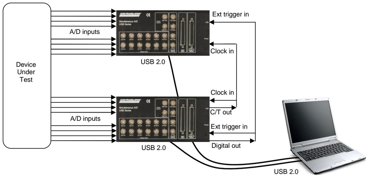
**Figure 1: Synchronizing two modules.**
