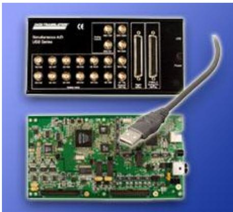
Data Translation application engineers proposed a unique answer that the manufacturer would not have thought of: Use two DT9836-12 high-performance, isolated simultaneous data acquisition USB modules in tandem. The modules use the USB 2.0 bus, which is readily available on the notebook
