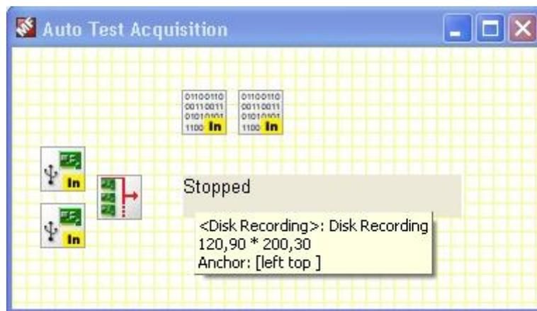
**Figure 2:** In Measure Foundry design mode, two Analog Input components, left, combine data in a Signal Synchronizer component. Data is captured with the Disk Recording component (shown with tooltip). The two Digital Input components provide triggering. Components are connected through configuration on property pages. During runtime, only the Disk Recording component will appear.
