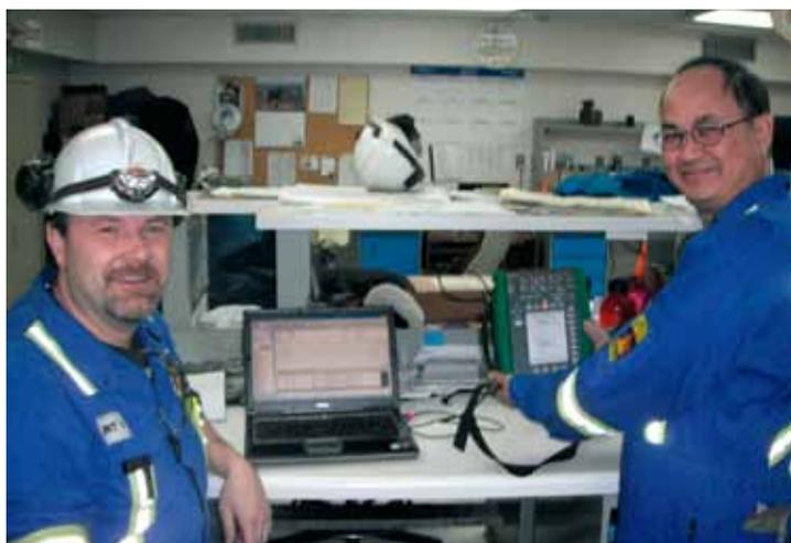
During a shutdown and turnaround all the plant instruments have to be calibrated for specific processes.
