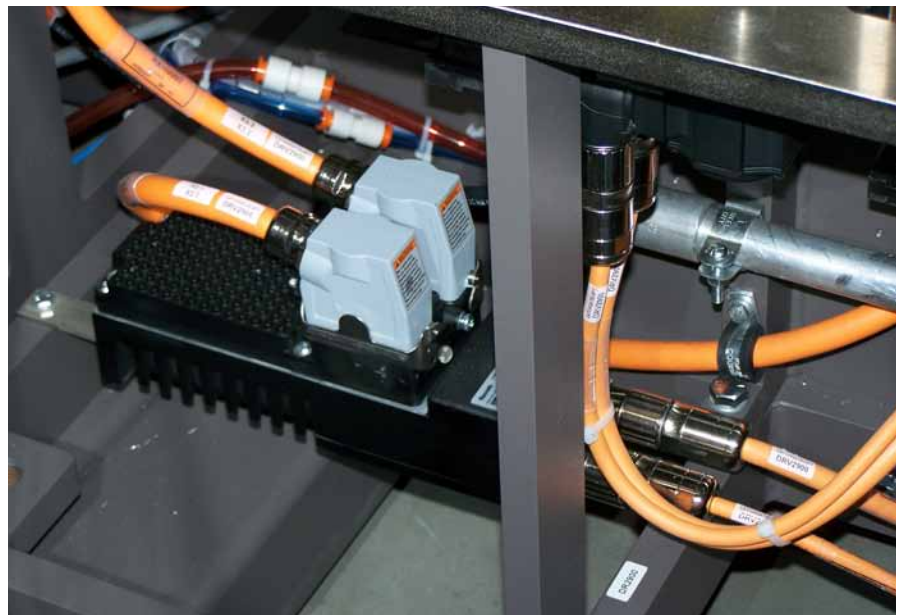
The IndraDrive Mi has the potential to reduce a machine’s cabling needs by more than 80%.
