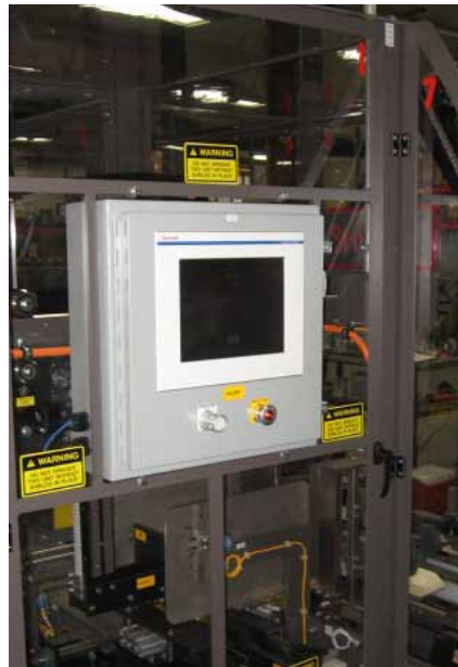
Mounted on the machine frame, the Rexroth IndraControl HMI uses a Windows CE-based platform and integrates easily with the rest of the control system.
