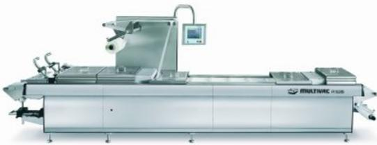
*Photo: A motor-gearbox combination achieves a bonding pressure of 20 tons in the high performance R535 packaging machine. Being a strategic motion control partner for Multivac, Kollmorgen implemented a compact unit of their AKM servo motor series and a cycloidal gear drive for the lifting axis. The high power density of this unit allows for compact dimensions.*
