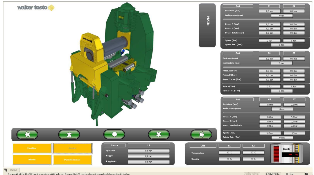
The supervision system which controls the world's biggest calender machine is based on Movicon 11.
