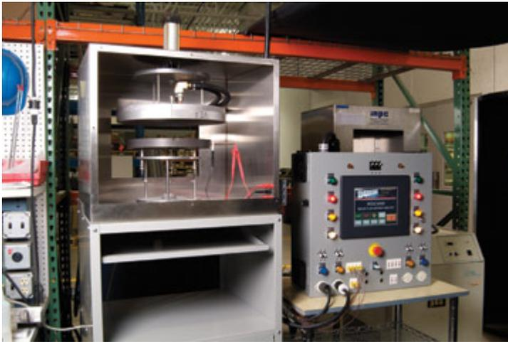
This test station needed a user-friendly graphical interface to give operators the ability to select multiple ramp/soak parameters, output voltages, temperature sensor types, amperage ratings and total cycle counts on tests for the cast-in electric heater platens. The system also needed to record temperature, volts, and current draw throughout the test for use in quality reports.
