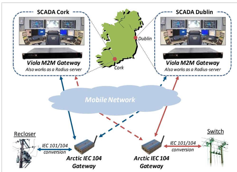
Figure 2: Fault-tolerant connections with Arctic devices
