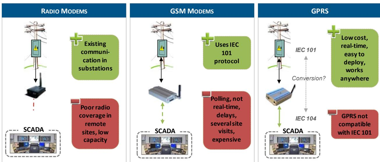
Figure 1: Communications gap - Comparing radio modems, GSM and GPRS
