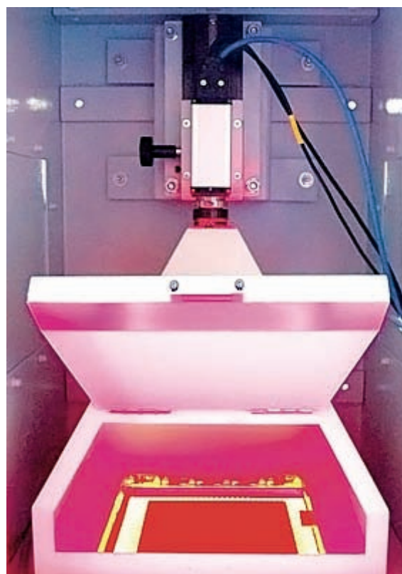
The uEye with 5 MP sensor captures even the tiniest cracks in a wafer under backlighting
