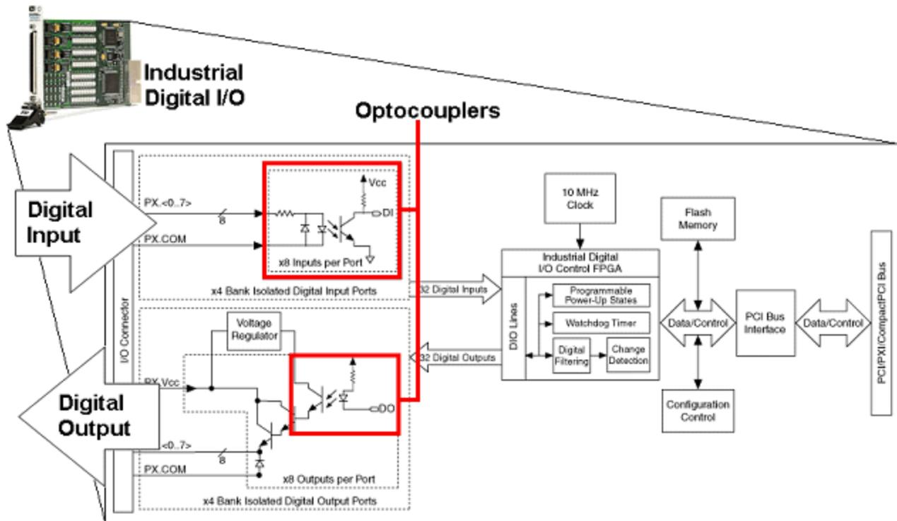
Figure 10. Industrial Digital I/O Products Use Optocouplers
