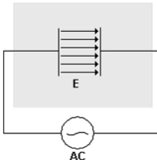
Figure 4. Capacitive Isolation
