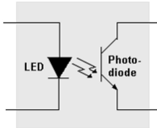
Figure 3. Optical Coupling
