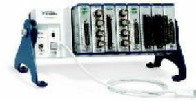
NI CompactDAQ – Modular USB data acquisition system with isolated input/output modules
