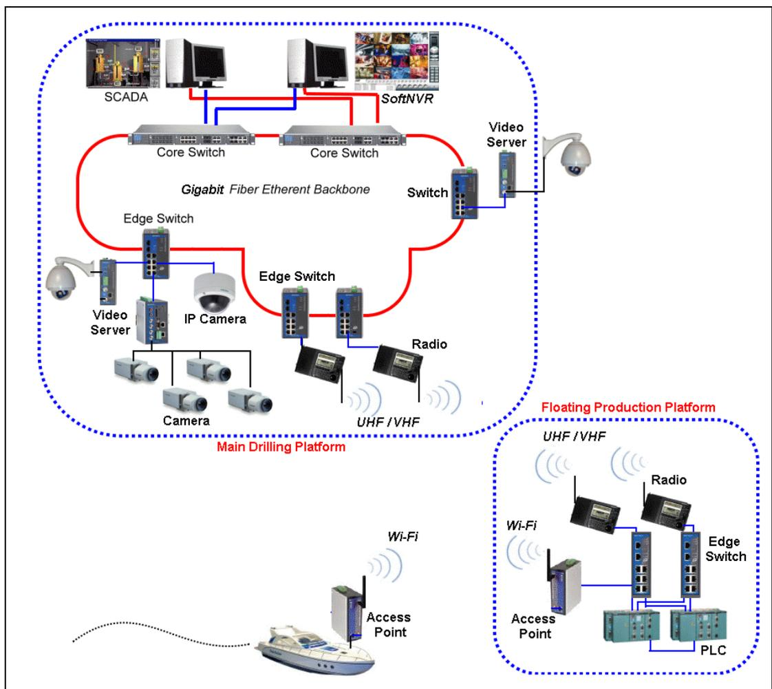
**Drilling Platform Communication & Video Solution**
