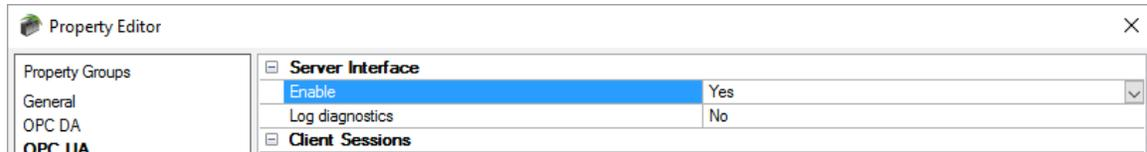
Then, define the OPC UA endpoint that represents TOP Server to OPC UA clients (similar to an OPC ProgID for OPC DA clients). This includes the level of secure encryption you wish to be enabled for this specific endpoint (this can sometimes be determined by the level of encryption your OPC UA client actually supports).
