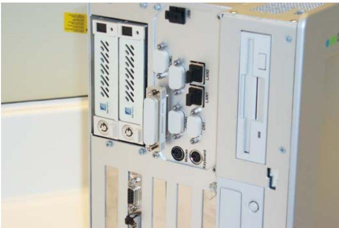
Figure #5, Industrial PC with dual RAID hard drives
