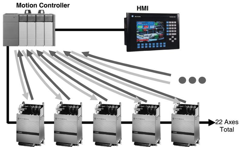
**Figure 2. Centralized Motion Control.**
