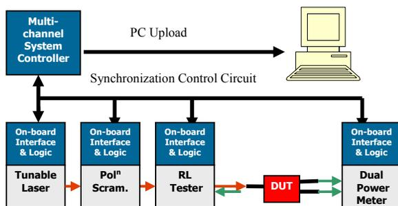
In contrast, the USB-inSync system (Figure 5) does not require a dedicated system controller, industrial backplane or on-board user interfaces and control logic. This is now handled by the PC and standard USB expansion bus. All logic control, software analysis and user interface components are now in the PC itself.
