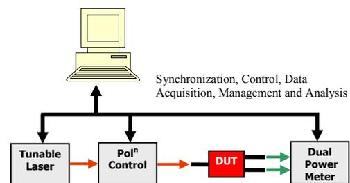
This scenario would involve measurement of insertion loss with a swept laser at four discrete states of polarization and then performing a numerical approximation based on Matrix mathematics to reveal PDL at each of the sampled wavelengths.
