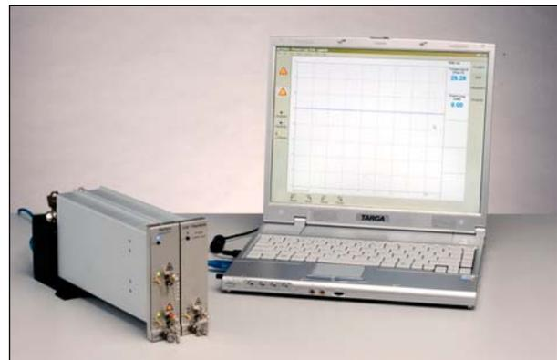
**Figure 3: Synchronized PC control of multiple test devices via USB-inSync**
