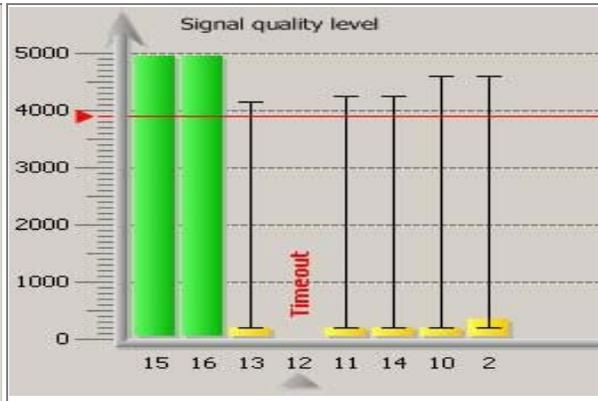
Correct evaluation of Signal level after removing bus termination
