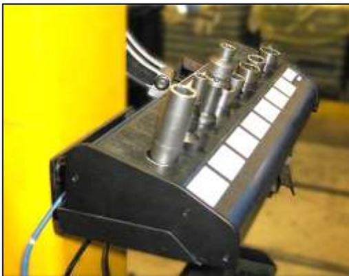
*Figure 3: Socket verification system.*
