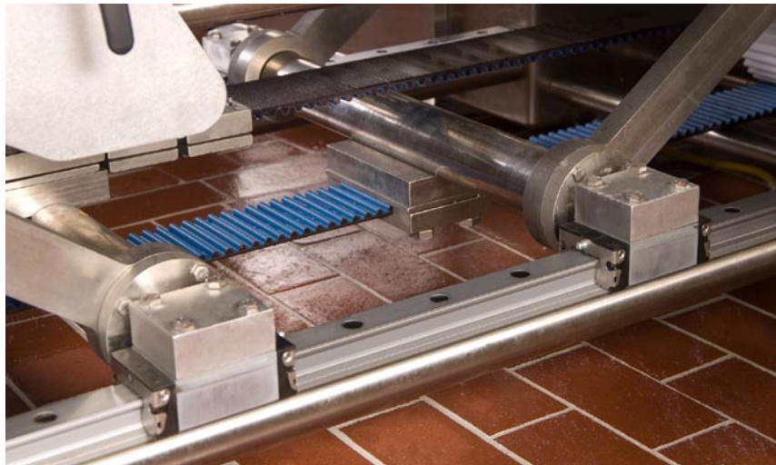
CP's unique synchronized belt-driven motion and lift system rides on Rexroth linear Ball Rails.
