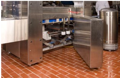
Motion and logic is controlled by a Rexroth SERCOS-based IndraMotion MLC controller with built-in motion, logic, robotic and Flex Profile capabilities—located in the unique swing-out control cabinet.
