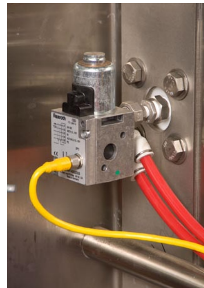
The Rexroth HF03-LG modular valve manifold system provides high flow in a compact package, while the ED05 electro-pneumatic proportional valve replaces the mechanical dancer on the film rollers.
