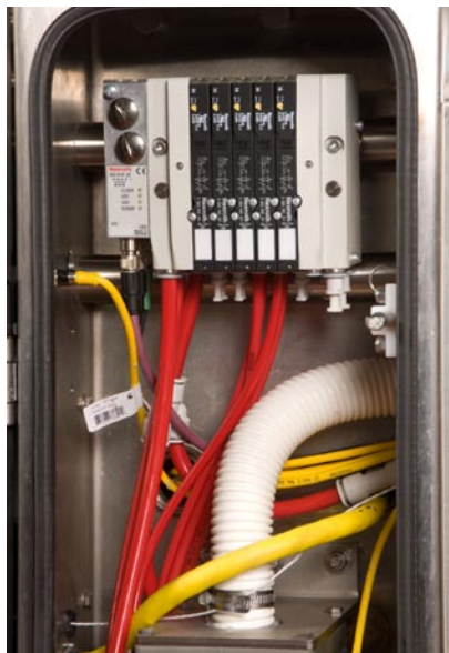
The Rexroth HF03-LG modular valve manifold system provides high flow in a compact package, while the ED05 electro-pneumatic proportional valve replaces the mechanical dancer on the film rollers.
