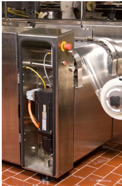
Rexroth IndraDrive Mi integrated motor and drive units are located directly on the machine, saving on wiring and cabinet space and enhancing sanitation.
