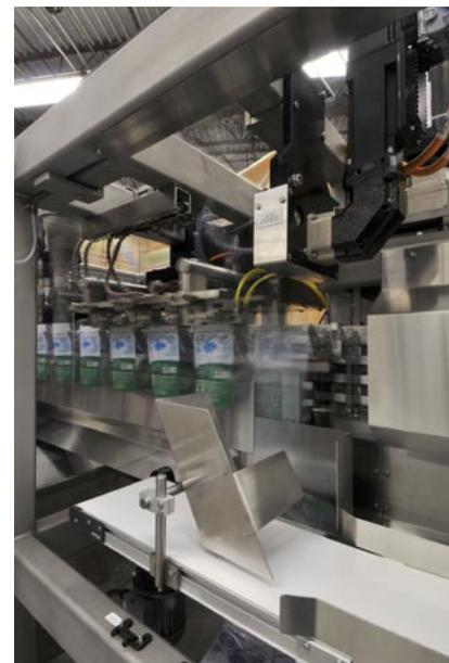
With the Rexroth servo and pneumatic system, KHS was able to build in better flexibility for timing, the ability to make changes on the fly, link functions together and provide quicker set-up and changeover time.
