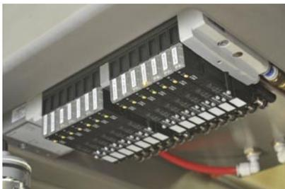
Instead of valves mounted all over the machine, KHS uses one Rexroth HF03-LG valve bank that can distribute air throughout, which reduces wiring and is expandable for more functionality.
