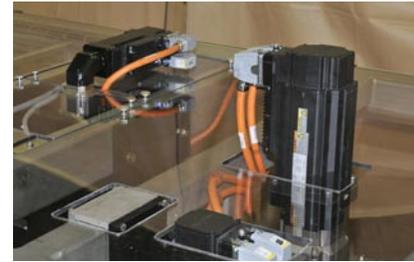
With the IndraDrive Mi, the daisy chain approach to wiring helps with the modular aspect KHS wanted, as well as adding to the clean design of the machine.
