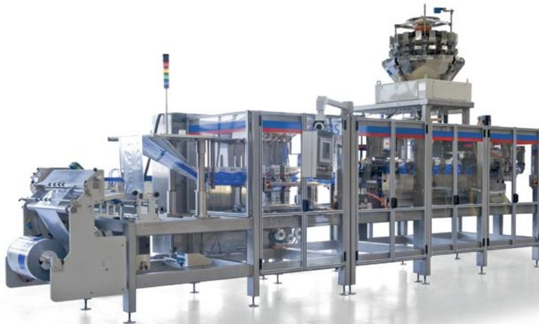
Rexroth provided a drive and control system for the KHS Innopouch K-series, a modular, flexible pouching machine with fast setup and changeover times and the ability to expand easily as needed. *(photo credit: KHS)*
