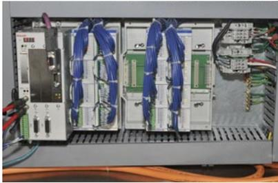
Machine control is provided by a high-performance Rexroth PPC-R controller with built-in motion, logic and robotic capability.
