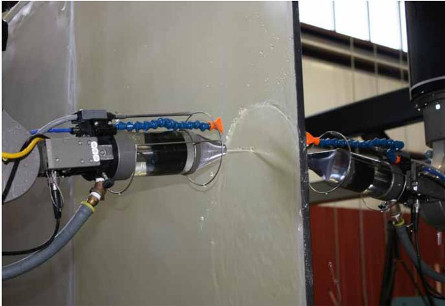
easily be configured to test a wide range of parts for each customer, instead of being designed for one specific part. The scanner's ultrasonic scanning system utilizes two sets of squirter jets that face each other. During inspection, the jets stream water—the medium that the sound wave travels through—around the part.
