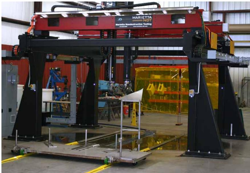
The gantry style AG2 Overhead Scanner is capable of scanning large, sophisticated parts and intricate shapes, without the use of immersion tanks.
