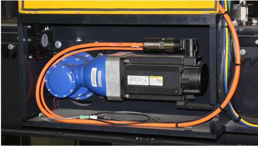
Servo motors like the IndraDrive MSK, along with Rexroth L65 servo controllers, provide precise positioning on the AG2's 16 axes of motion.
