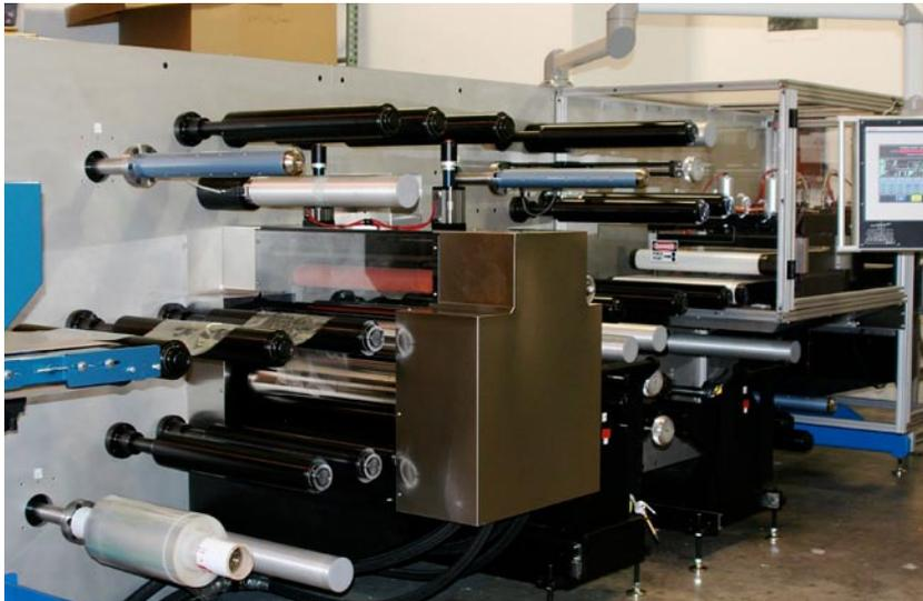
Using a Rexroth control system, Summit's web converter is a 20-axis converting machine that takes material compounds and precisely forms them against a substrate to create the final product.
