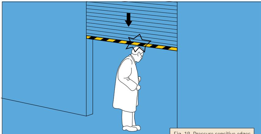
Fig. 18 Pressure sensitive edges
