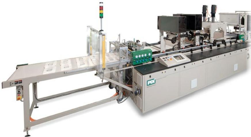
The PDI Medical Combination Pouch System uses a Rexroth control system to convert pre-made medical header bags and shaped pouches to exacting industry specifications at a rate of nearly 200 seals per minute.
