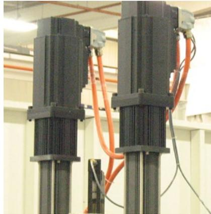
The IndraDrive Mi integrated servo motor/drive allows for precise control with a smaller machine footprint and a significant reduction in cabling and installation costs.
