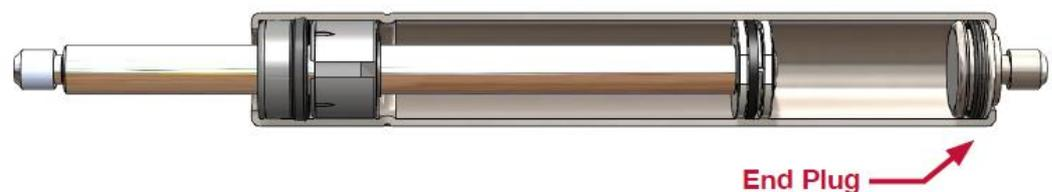
The end plug is used to seal the tube end of the gas spring, with this also attaching to the tube end fitting. Camloc's Vari-Lift™ can be incorporated here where required, allowing for the release of Nitrogen gas and subsequent reduction in force of the spring.
