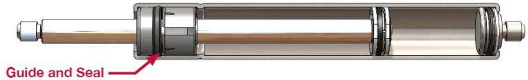
Manufactured from plastic composite, the guide and seal package provide a bearing surface for the rod and prevents the escape of gas and ingress of contamination.
