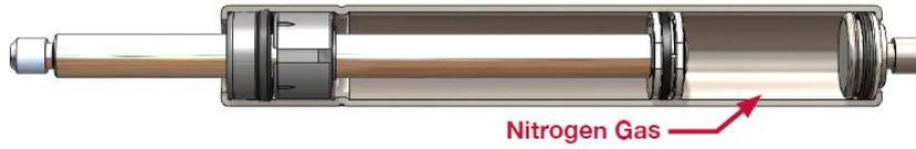
Nitrogen is used inside gas springs as it is inert and non-flammable, therefore not reacting with any of the internal components.
