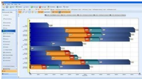
Condition monitoring software allows users to visualize data from many distributed machines at once, and to analyze this data to identify faults before they can further develop and cause downtime.
