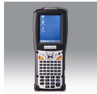
The operator can use the handheld's display to serve as an auxiliary HMI terminal and make
