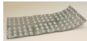
Empty wells appear dark and are easily detected by the vision system
