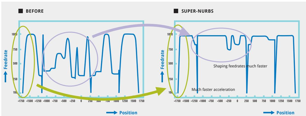
it will create a spline that is a “best fit” and may eliminate some of the points that are redundant to the spline path. This allows for a smoother tool path, and because we eliminate some of the points, the positioning feedback does not need to crunch as much data and can speed up the movements while still maintaining accuracy.
