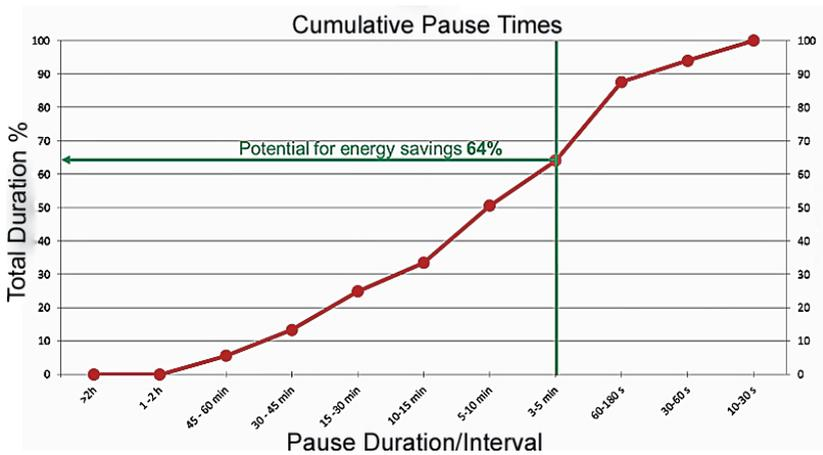
**Idle time distribution: pauses of less than 5 minutes may not be exploitable**
