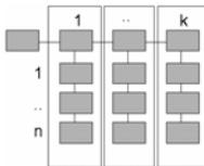
**Comb structure:** Main line with  $k = 8$  stations in every bus cycle; plant components with  $n = 10$  users in every 8th cycle; distance between users = 50 meters in both cases.
