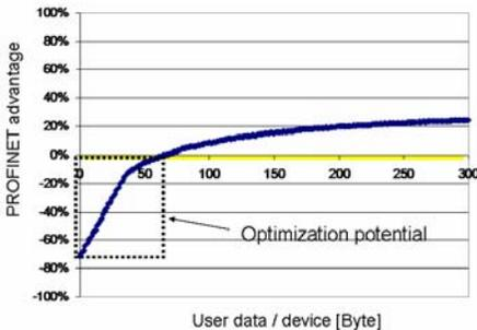
**Line structures:** Here, it was shown that PROFINET has the advantage for larger data packet sizes. However, at smaller packet sizes, the 'summation frame' approach reacts faster.
