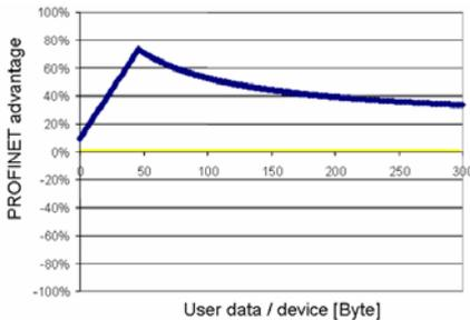
**'Comb' structures:** Here, it was shown that PROFINET reacts more flexibly and faster across virtually the entire case spectrum with, broadly, a 40% speed advantage. In comb structures, 'summation frames' always have to go through each node twice (they have to follow the branches out and back
