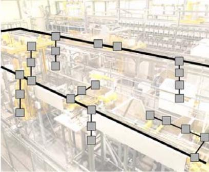
Modern manufacturing plants are typically based on a combination of line and branch network structures. This is because a factory floor often requires many production units to be linked together, while the individual units themselves have localized needs based on the requirements of the process and the machine or cell design.
