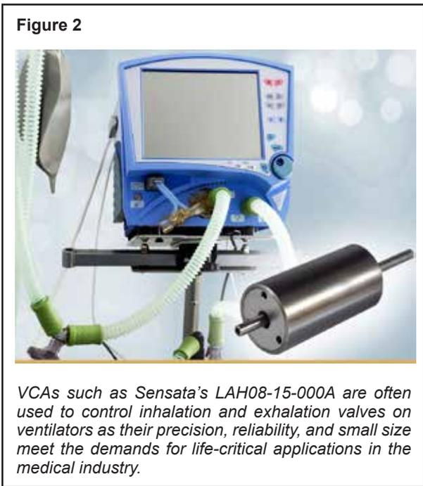
Another advantage with of these types of VCA motors are their bi-directional capabilities, permanent magnets, and magnetic latches, enabling the VCA to remain in position at one end or the other of a stroke during a power failure, ensuring the valves stay open or closed in a disruptive power situation.
