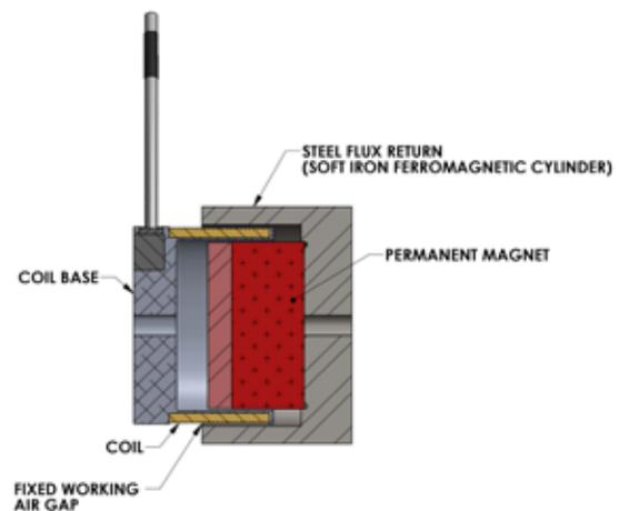
*Used in a wide range of medical and industrial applications, an axial voice coil actuator is composed of a permanent magnet situated within a moving tubular coil of wire, all inside of a ferromagnetic cylinder. When current runs through the coil, it becomes magnetized and repels against the magnets, producing an in and out, back and forth motion.*
