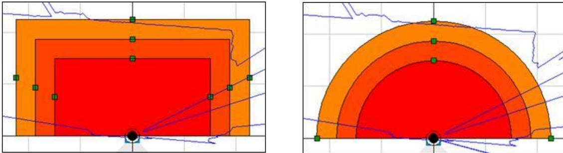
**Active laser scanner sensing devices offer rectangular or radial zones of configurable size.**
