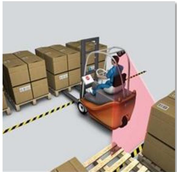
The laser scanners that are easiest to implement include push button control for easy teaching of detection areas, or zones. This means the user defines the dimensions of warning (and/or stopping) zones interactively—by putting the scanner in “teach mode” and walking the desired field’s shape in front of the scanner. Alternately, zone programming can be drawn using a graphical interface integrated with the scanner’s control software.
