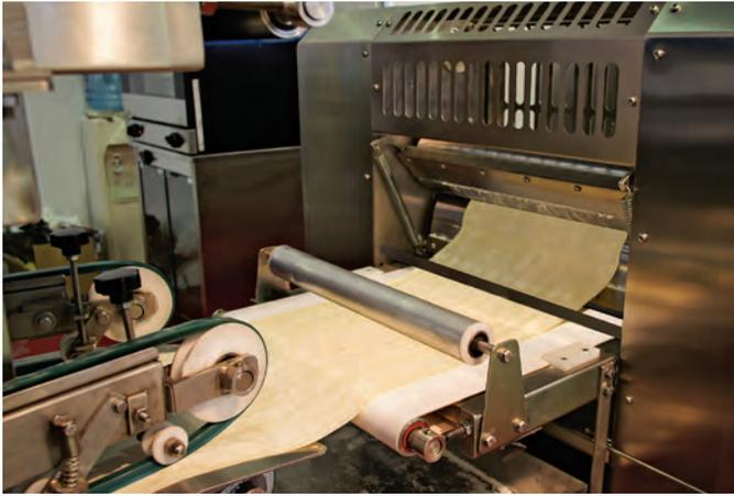
So much about chewing gum has remained timeless – its form, function, and appeal. One core function of gum-making machines has also remained timeless, and that is the process of kneading and shaping ingredients into sheets for cutting and packaging. Machines that manage this process are called sheeters. While their function has stayed constant, gum sheeters have evolved through innovation.
