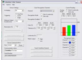
Color sensors are available with a wide variety of features ranging from simple teach functionality to a full featured GUI interface that allows real-time display, access to tolerance settings for each color and general sensor controls. While simple applications such as sorting based on a few very different colors can often be accomplished with the lower end color sensors, many others will require more comprehensive control of settings provided by the full-featured sensors.
